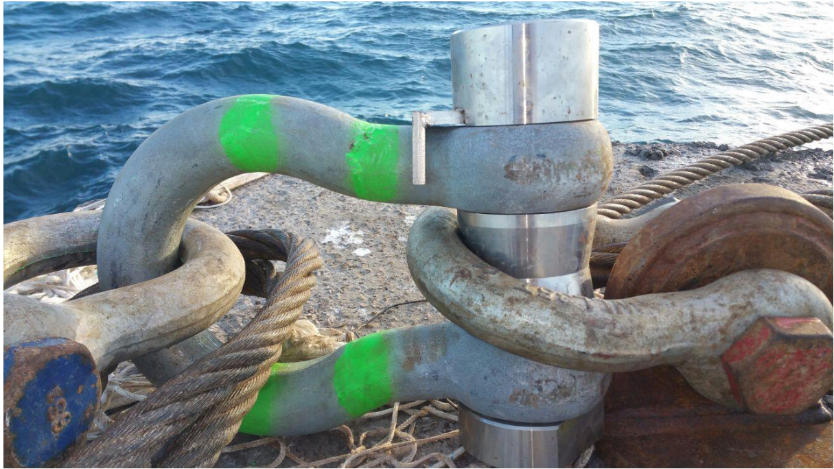
Figure 4-6. 75 ton load shackle [21].
